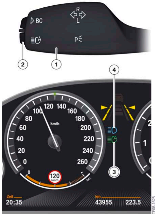
F10 High-beam assistant display and button
